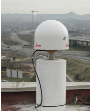
GNSS continuous operating reference stations
